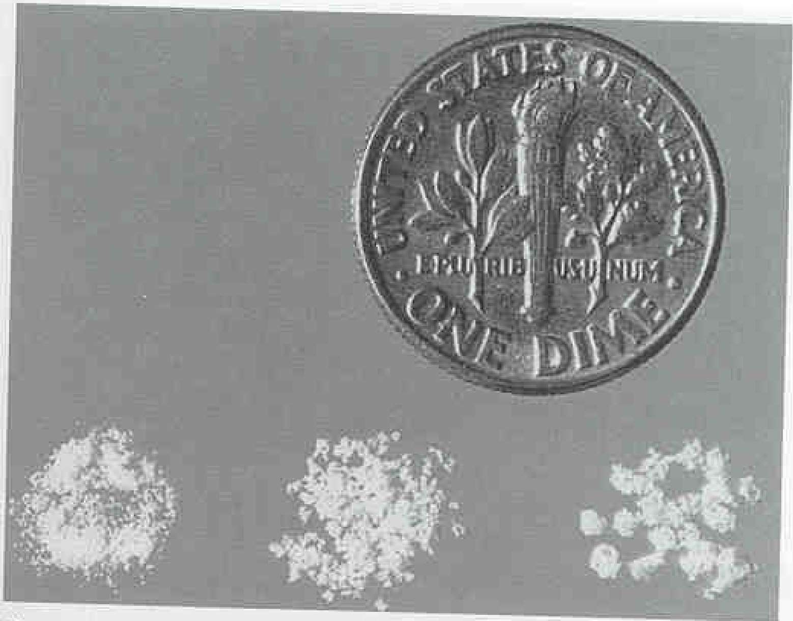
Figure 1-50 Sizing of PVA particles made by ITC/Target Therapeutics (Contour Emboli). Note the irregularity of the particles themselves.
